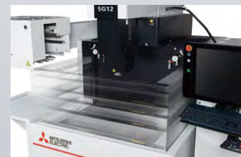
3-sided automatic elevation working tank
