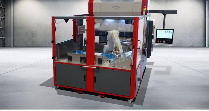
The **SMARTFLEX Mobile Bending Cell** features the compact yet powerful Mitsubishi RV13 robot and lightning-fast Diamond BB Series electric press brake. You'll be fully equipped for lights-out bending - four infeed trays have a generous 13.3 square feet for part loading. The press brake can be run during the day for complicated parts, then equipped with the mobile cell for on-demand lights-out bending of simpler parts or high runners.
